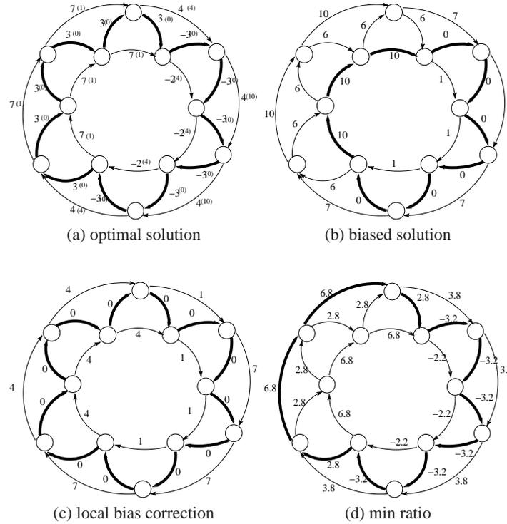
**Fig. 4.** Bold lines indicate the optimal contour. In (a) the weights in parentheses are obtained by optimally converting the negative weights to positive. Graph (b) is obtained by adding 3 to the original weights of graph (a). In (c) the local bias correction is applied to the weights of (b). In (d) the weights of (b) are transformed according to the min ratio cycle method.
