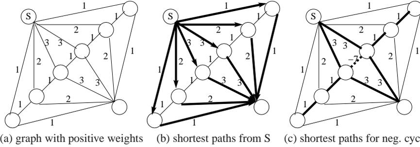
**Fig. 2.** Negatively weighted cycles act as black holes in the energy landscape. (a) Original graph with positive weights. (b) Shortest paths from  $S$  to all the other nodes for the weights of (a) (shown with bold arrowed lines). (c) The edge indicated with dashed line has obtained negative weight  $-7$  and negative cycles have been created. The shortest path from  $S$  (shown with bold lines) are forced to include such cycles.
