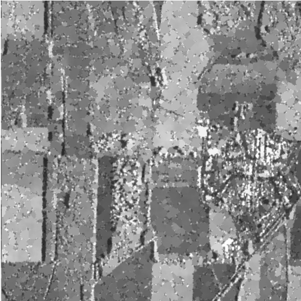
Figure 12: Region-based GGMAP speckle filter exploiting segments shown in Fig. 11.
