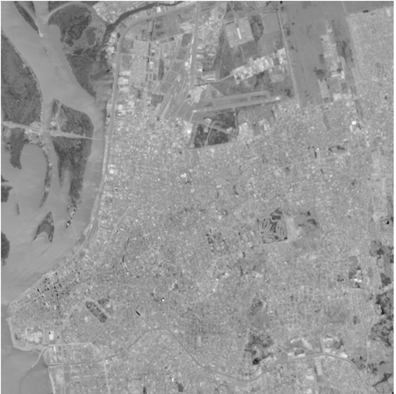
Figure 15: SPOT HRV image of the city of Porto Alegre (Rio Grande do Sul, Brazil): Band 1 (Visible Green; 512x512 pixels).
