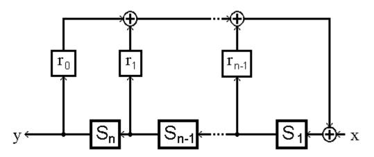
An n-SA is said to be **degenerated** if it holds  $\mathbf{r}_0 = 0$ , and **non-degenerated** otherwise. Moreover, the 'extremely degenerated' n-SA without any feedback connection (i.e.  $\mathbf{r}_i = 0$  for i = 0,...,n-1) will be referred to be the **trivial** n-SA. In most cases, however, only non-degenerated SAs will be considered.
