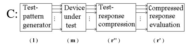
In this figure, the right component ( $\mathbf{r}$ ) from the original picture  $\mathbf{T}$  has been changed into a similar device ( $\mathbf{r'}$ ). The new device, however, does not evaluate the complete test response sequences but only the result of some data compression. This compression will be performed by the completely new component ( $\mathbf{r''}$ ) which is not contained in the figure  $\mathbf{T}$  but which is now directly connected to the output lines of the DUT.
