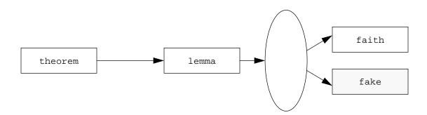
FIGURE 7. Logical topology of the local testbed. For some experiments, additional network load was created on lemma's outgoing interface by sending additional network traffic to a non-existent machine (fake), shown in the shaded box.
