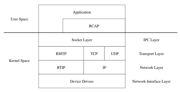
FIGURE 5. Software structure of RMTP/RTIP. The Internet protocols co-exist with the Tenet Suite.
