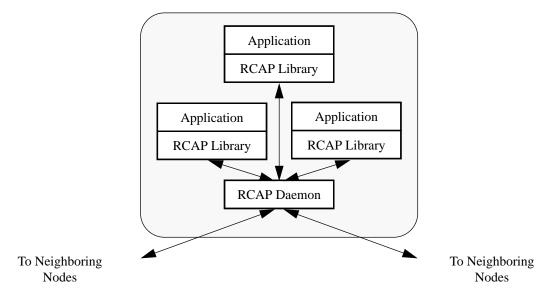
FIGURE 4. The RCAP library and daemon, within a single network node. Arrows represent RCAP control connections.
