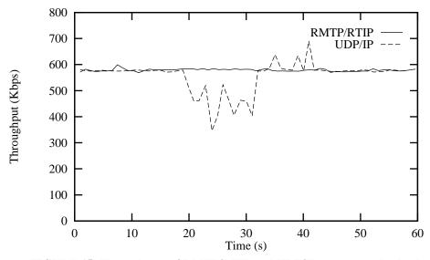
FIGURE 15. Throughputs of RMTP/RTIP and UDP/IP streams under load.
