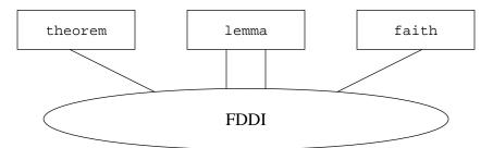
FIGURE 6. Physical topology of the local testbed. theorem and lemma are DECstation 5000/125s and faith is a DECstation 5000/240. Note that lemma has two FDDI interfaces. All machines run the Ultrix 4.2A operating system.
