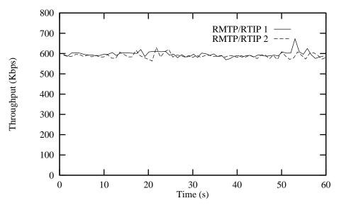
FIGURE 16. Throughputs of co-existing RMTP/RTIP channels.
