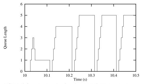
FIGURE 13. Queue length vs. time, for a single RMTP/RTIP channel under congestion.
