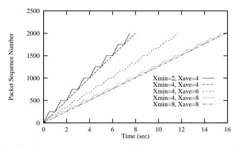
FIGURE 10. Effect of rate control at source on an RMTP/RTIP channel. The source process is attempting to send packets in a tight loop, but its rate is limited by the rate control mechanism.
