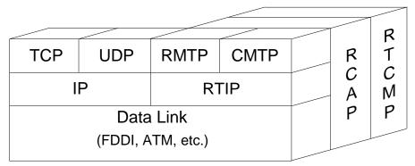
FIGURE 1. The Tenet Real-Time Protocol Suite. Also shown are the corresponding Internet protocols.
