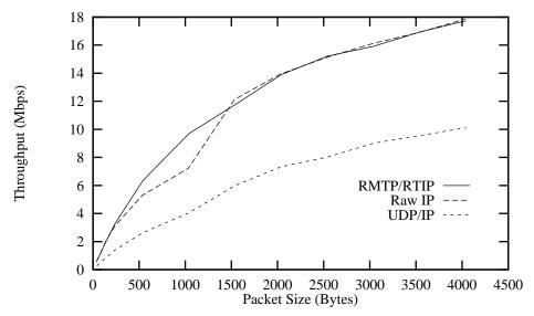
FIGURE 8. Throughput of RMTP/RTIP, UDP/IP, and raw IP.
