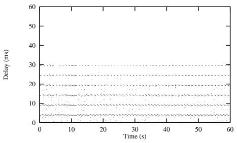
FIGURE 14. Packet delays over times, for a single RMTP/RTIP channel under congestion. The mean delay is 7.37 ms.
