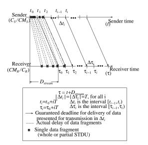
Figure 2.3: Timing diagram for Continuous Media Transport Service
