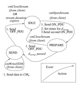
Figure 5.4: Channel state transitions at  $CM_S$  (data connection only)
