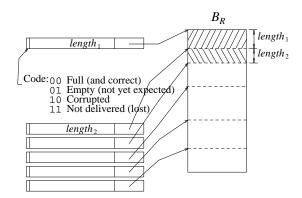
Figure 6.2: Shared buffer with descriptors (receiver shown)
