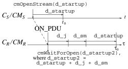
Figure 6.3: Timing diagram of start of stream
