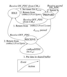
Figure 5.5: Channel state transitions at  $CM_R$
