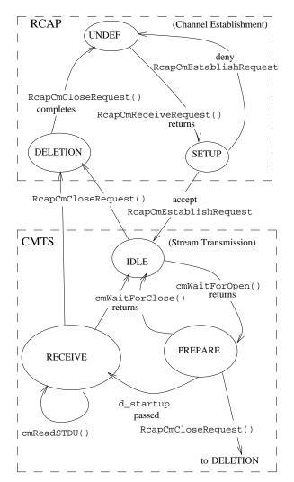
Figure 4.2: Transitions of channel state at the receiver
