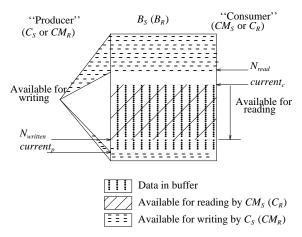
Figure 6.1: Conceptual view of shared circular buffer
