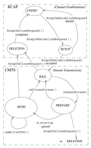
Figure 4.1: Transitions of channel state at the sender
