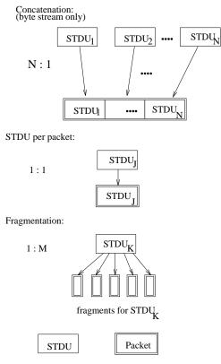
Figure 5.2: Mapping of STDUs into packets (DATA\_PDUs)
