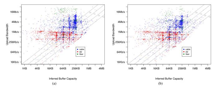
Figure 3: Uplink buffering as observed for wired (a) and wireless (b) hosts for major ISPs where we can classify the link technology used in the connection.
