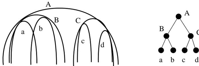
Figure 2: A bump tree for holding Gaussians.
