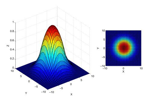
Figure 11: Radially quadratic B-spline function (Eq. 67).
