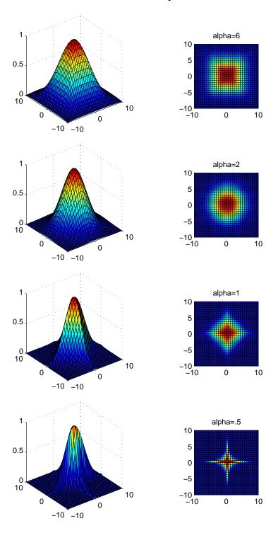
Figure 3: Gauss function with different Minkovski norms.
