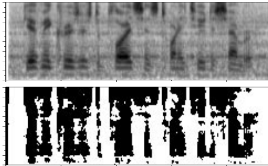
Figure 7: The upper panel shows an auditory spectrogram for the utterance “GIVE ME CRUISERS DEPLOYED SINCE TWENTY TWO DECEMBER” mixed with Lynx helicopter noise at a global SNR of 18 dB. Dark regions of the lower panel indicate those areas where the local SNR is positive. Attempts to recognize the mixture with a conventional recognizer yielded “IS HORNE+S FOUR DECEMBER” while use of first-generation missing data techniques via the lower mask produced “GIVE CRUISERS DEPLOYED SEVENTH DECEMBER”.
