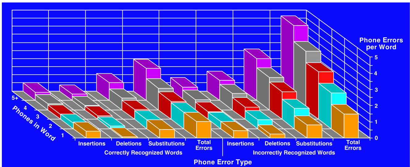
Figure 7: The number of phonetic-segment errors per word as a function of the number of phones contained in the word. The data are partitioned into two broad classes - correctly and incorrectly recognized words. Within each subset the data are divided into four classes, based on the type of error. Data represent averages across the eight ASR systems. Words of designated length "5+" contain five or more phones.
